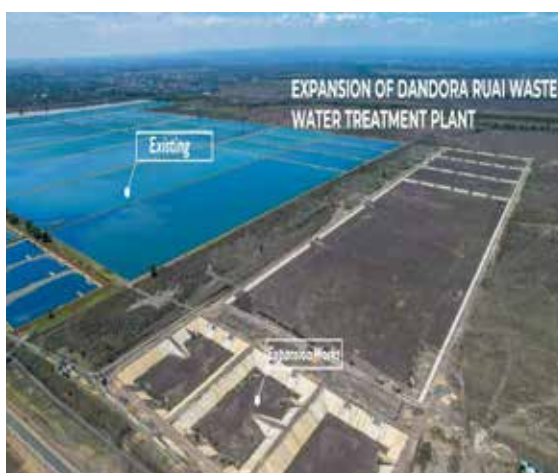
Dandora Estate Sewerage Treatment Plant features the largest wastewater stabilization pond in Africa, treating 80,000 m 3 of sewerage per day (80% of Nairobi's wastewater)
